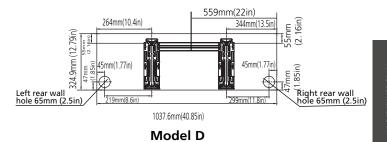
**NOTE:** When the gas side connective pipe is  $\Phi$  16mm(5/8in) or more, the wall hole should be 90mm(3.54in).
